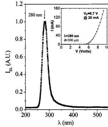
FIG. 2. EL spectrum of a disk shape ( $d=300 \mu\text{m}$ ) deep-UV LED with peak emission at 280 nm under dc bias ( $I=40 \text{ mA}$ ). Inset is the  $I$ - $V$  characteristic of the same 280 nm UV LED.
