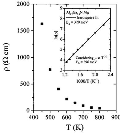
FIG. 1. Temperature variation of resistivity of a Mg-doped  $\text{Al}_{0.7}\text{Ga}_{0.3}\text{N}$  epilayer in the temperature range of 450–800 K. Inset is the semilog plot of  $\rho$  vs  $1/T$ . The solid line is the least-square fit of data with Eq. (1). The fitted value of  $E_A$ , the activation energy of Mg acceptor is 320 meV (396 meV) without (with) considering the variation of  $\mu$  with  $T$  ( $\mu \propto T^{-3/2}$ ).
