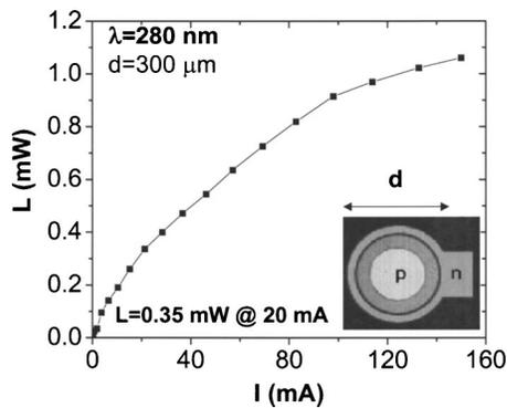
FIG. 3. ( $L$ - $I$ ) of a circular ( $d=300\ \mu\text{m}$ ) deep-UV LED (280 nm). Inset is an optical microscope image of the fabricated LED.
